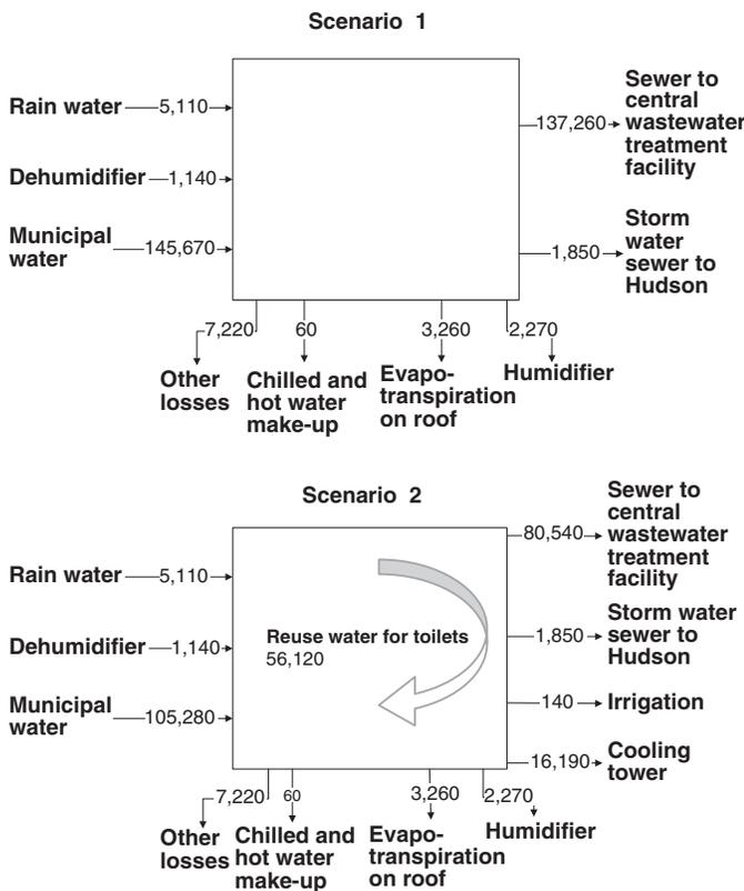
FIGURE 3. Summary Water Mass Balance for Solaire Scenarios (Excluding the Cooling Tower and the Public Bathroom) for the Time Period From October 1, 2004, Until September 30, 2005 (l/d, Scenario 1: conventional building, Scenario 2: Solaire building).
