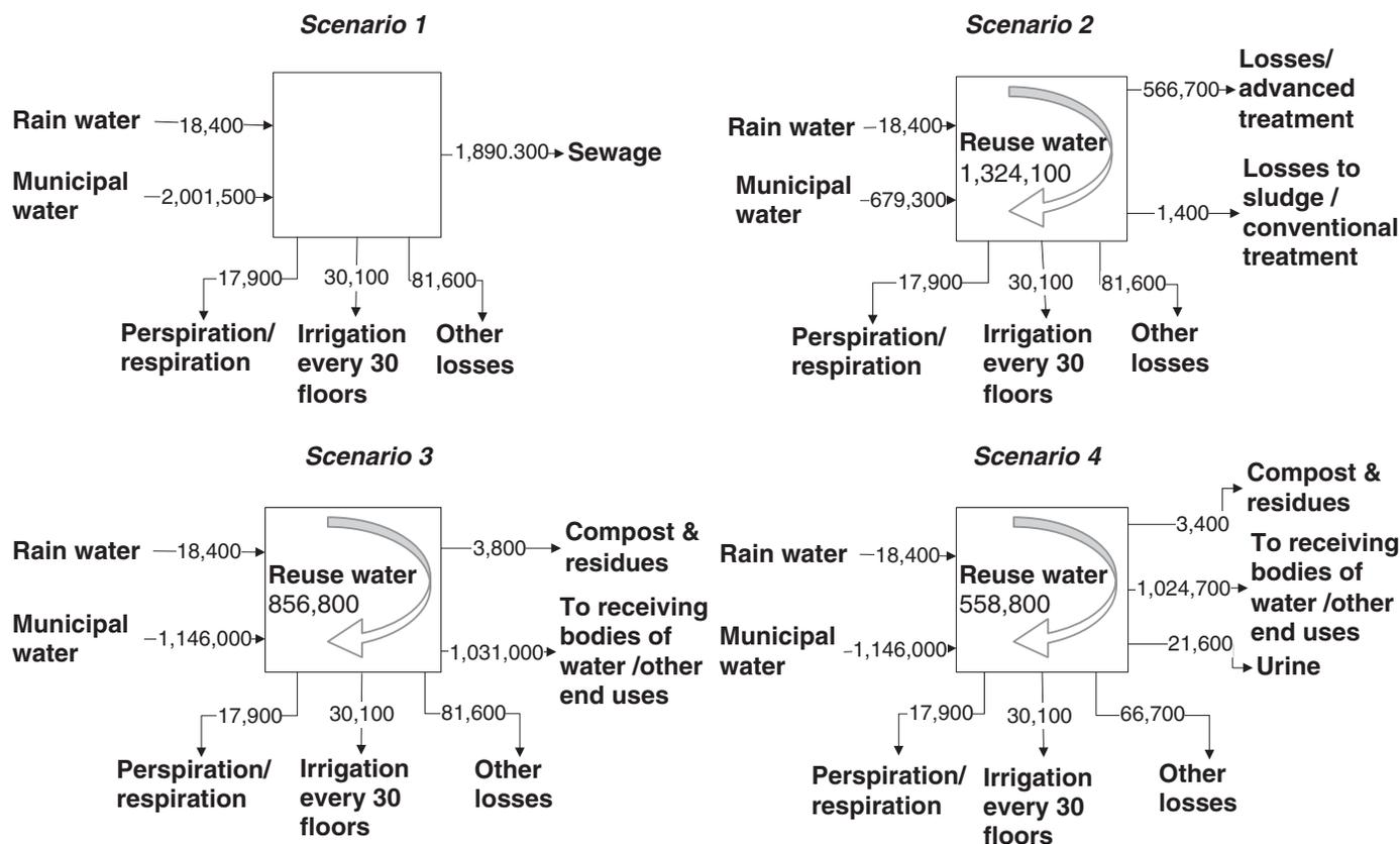
FIGURE 4. Water Mass Balances for 2020 Tower Scenarios [l/d, Scenario 1: conventional building; Scenario 2: 2020 Tower with treatment of wastewater to potable water; Scenario 3: 2020 Tower with treatment of source-separated streams to nonpotable water; and Scenario 4: 2020 Tower with treatment of source-separated streams to nonpotable water and separation of concentrated nutrients (urine)].
